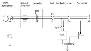
P1: main protective device of the installation
