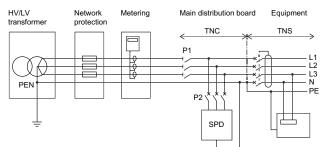
P1: main protective device of the installation P2: protective device used with the SPD (see 3.5.2) SPD: surge protective device
