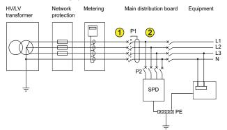
P1: main protective device of the installation P2: protective device used with the SPD (see 3.5.2) SPD: surge protective device
