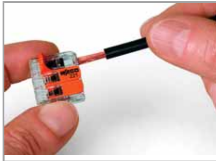
Termination: Lift the lever to open the clamping unit and insert a stripped conductor.
